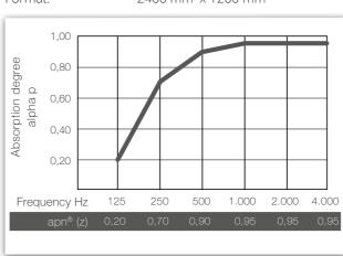
apn® Vinta (e) and apn® Vinta (eT) Structure height: 200 mm Format: 2400 mm x 1200 mm
